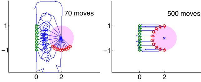
Fig. 4. Simulation set up. The  $n$  robots are initialized evenly spread between  $y = [-1, 1]$ , the goal is at  $(2, 0)$ , the nominal turn  $\phi = \pi/4$ , and the desired range and bearing to the target is  $(d, \alpha) = (1, 0)$ . Shown above are results for  $n = 10$  robots for different numbers of moves.
