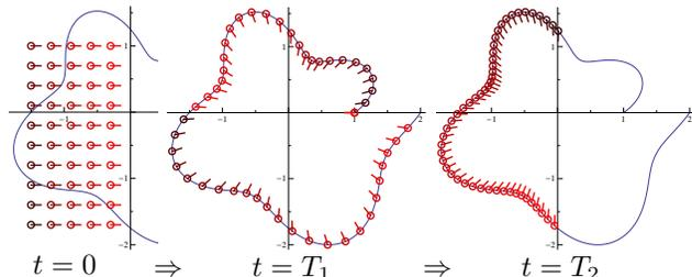
Fig. 1.  $n$  robots, under the constraint that each robot receives exactly the same control inputs, can be controlled from any initial configuration to the perimeter of a star-shaped set as long as each robot has a unique turning rate. The controller has  $2n + 1$  degrees of freedom, which can be used to permute the spacing around the perimeter (middle and right). See Section IV for details.
