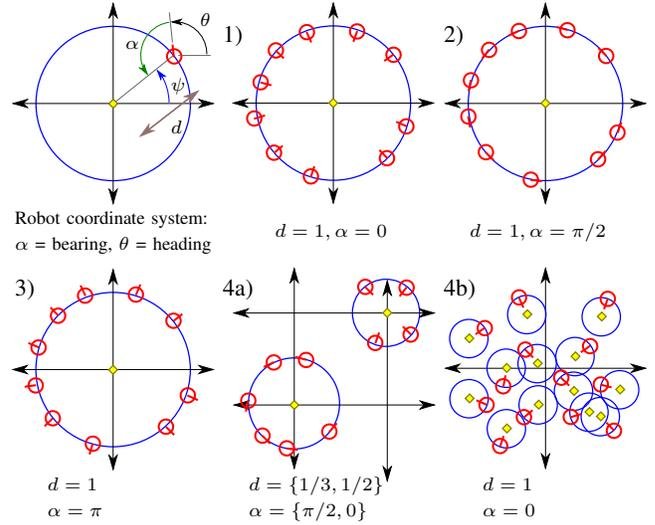
Fig. 3. Given  $n$  robots, where the pose of the  $i$ th robot is  $(x_i, y_i, \theta_i)$ , we can specify the desired bearing  $\alpha$  and range  $d$  for each robot to at most  $n$  targets at positions  $(x_{t,i}, y_{t,i})$ . Let  $\psi = \text{atan2}(x_i - x_{t,i}, y_i - y_{t,i})$ , then the heading  $\theta = \pi - \alpha + \psi$ .
