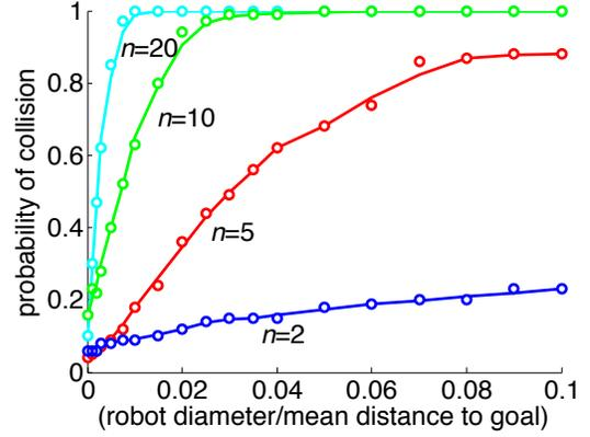
Fig. 6. Probability of a collision as a function of (robot diameter/mean distance to goal) for different numbers of robots,  $n$ . The setup in Fig. 4 is used. The probability of collision increases nonlinearly with number of robots and robot radius.
